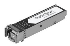
The 10056-ST is an Extreme Networks 10056 compatible downstream fiber SFP transceiver which pairs with StarTech.com's 10057-ST. They are designed, programmed and tested to work with 1000Base-BX-D compatible Extreme Networks switches and routers. The SFP transceiver module supports a maximum distance of up to 10 km (6.2 mi) and delivers dependable 1 GbE connectivity over fiber cabling.
